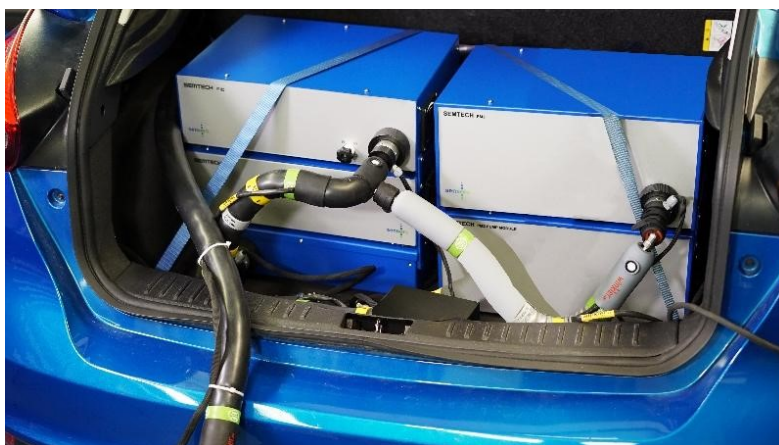
SEMTECH ® DS+ configuration shown with FID and PM2 modules
